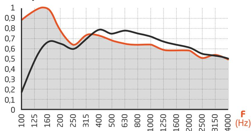
Medium acoustic absorption coefficient  $\alpha_m = 0,60$
