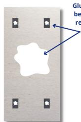
Glues or adhesives can be used for additional reinforcement of the clips or panel.
