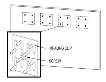
4. ENSURE PANEL IS LOCATED PROPERLY, PRESS PANEL FIRMLY TO WALL. (MAKE SURE THE FIBERGLASS CORE IS BEING IMPALED BY THE CLIPS, NOT THE FABRIC.)
