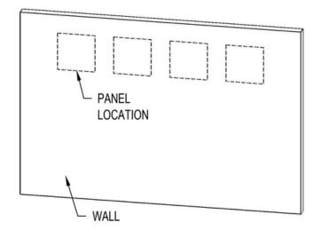
3. APPLY CONSTRUCTION ADHESIVE (BY OTHERS) TO FABRIC PERIMETER ON PANEL BACK. ADHESIVE BEAD SHOULD BE 3/4" x 3/4" x 6" LONG, NO MORE THAN 18" APART.
